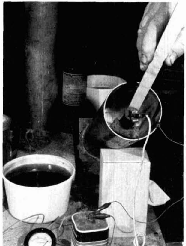
fig. 4. Silver plating the inside of the main tubing of a cavity.
