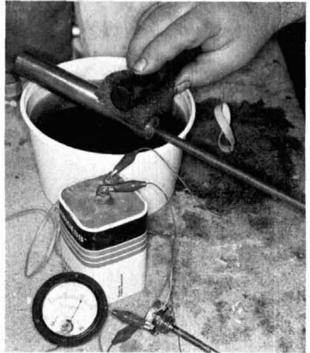
fig. 3. Silver plating the tuning rod of a cavity.
