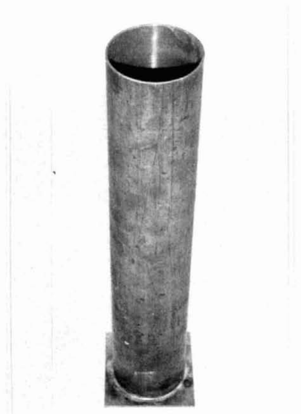
fig. 9. One of the six main copper tubes silver soldered to the bottom cover plate.
