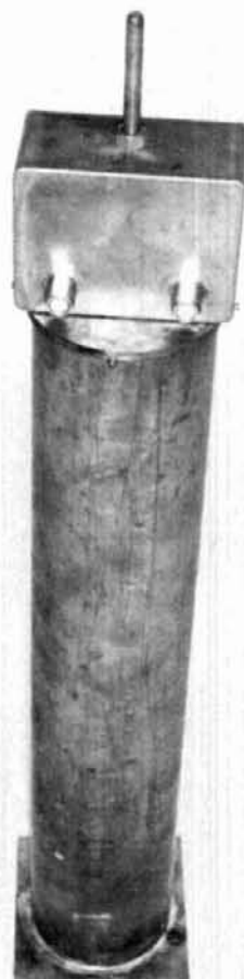
fig. 2. Completed cavity. Note the locking nut on the threaded rod to hold the tuning adjustment. Also note the metal chassis box, the two "N" type chassis connectors, top and bottom covers.
